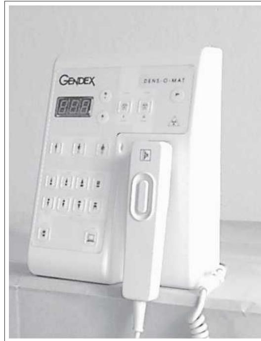
It also incorporates other circuits dedicated to safety functions such as back up timing, with independent monitor of the power line and stop of exposure if the maximum limit of 3.2 s. is exceeded.
