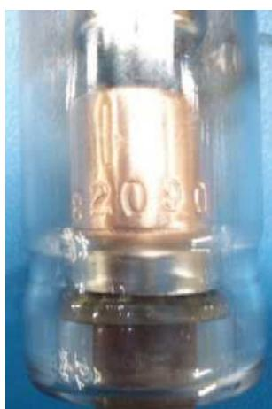
The serial number of the Gendex X-ray tube (PN 800-0003G3) is stamped on the copper anode of the tube assembly.
